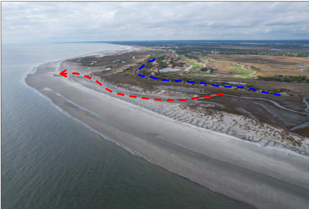
FIGURE 4.8. [UPPER] December 2024 and [LOWER] December 2025 aerial images of the Lagoon Reach. The blue dashed line is the approximate 1989 shoreline. As of December 2025, the east-end channel has shifted westward and mostly closed compared to December 2024 (red line).
