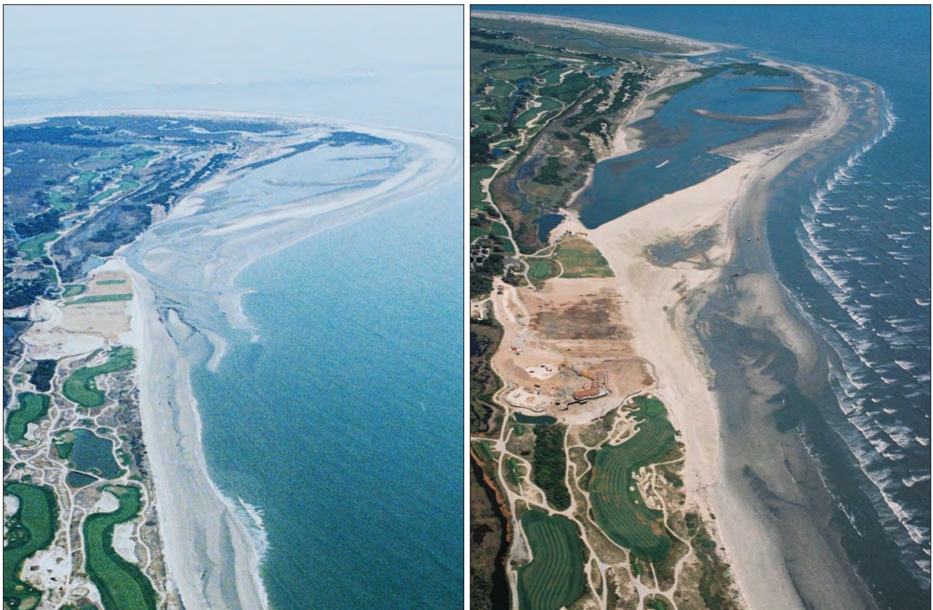
FIGURE 2.9. Before (February 2006) and after (July 2006) aerial photos of the 2006 East End beach restoration project. [After CSE 2007]
